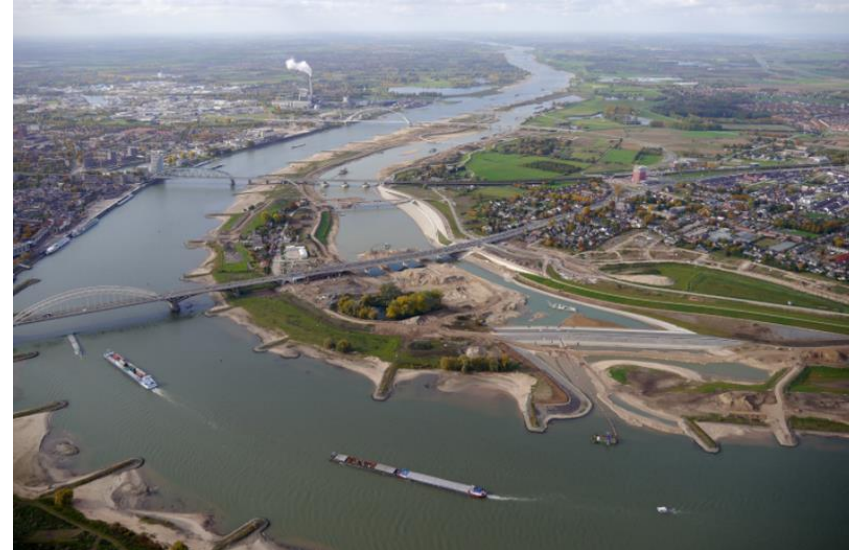
Room for the Waal River: Implemented interventions include the relocation of the Lent dike, the digging of a new river channel and the creation of a new island. Source: https://goexplorer.org/nijmegen-embracing-the-river-to-combat-flooding/
